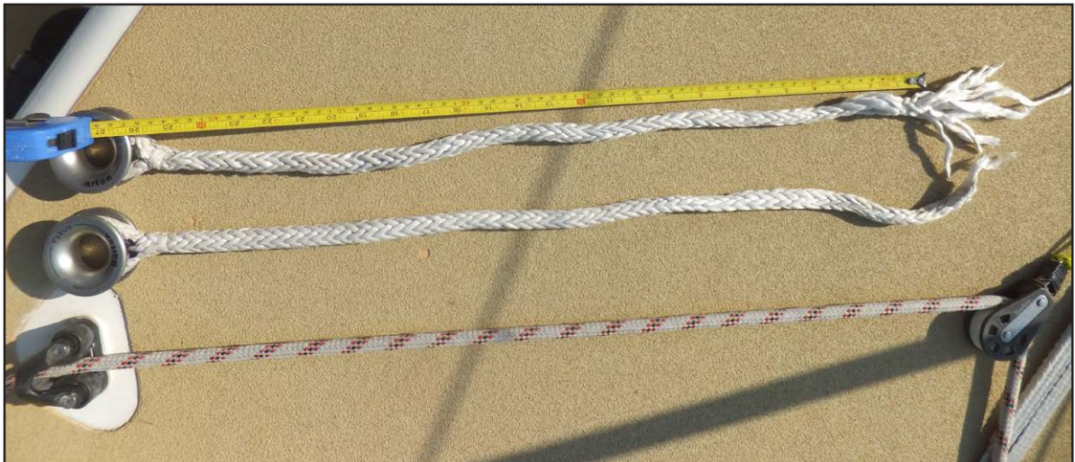
Figure 14: Failed preventer strop
