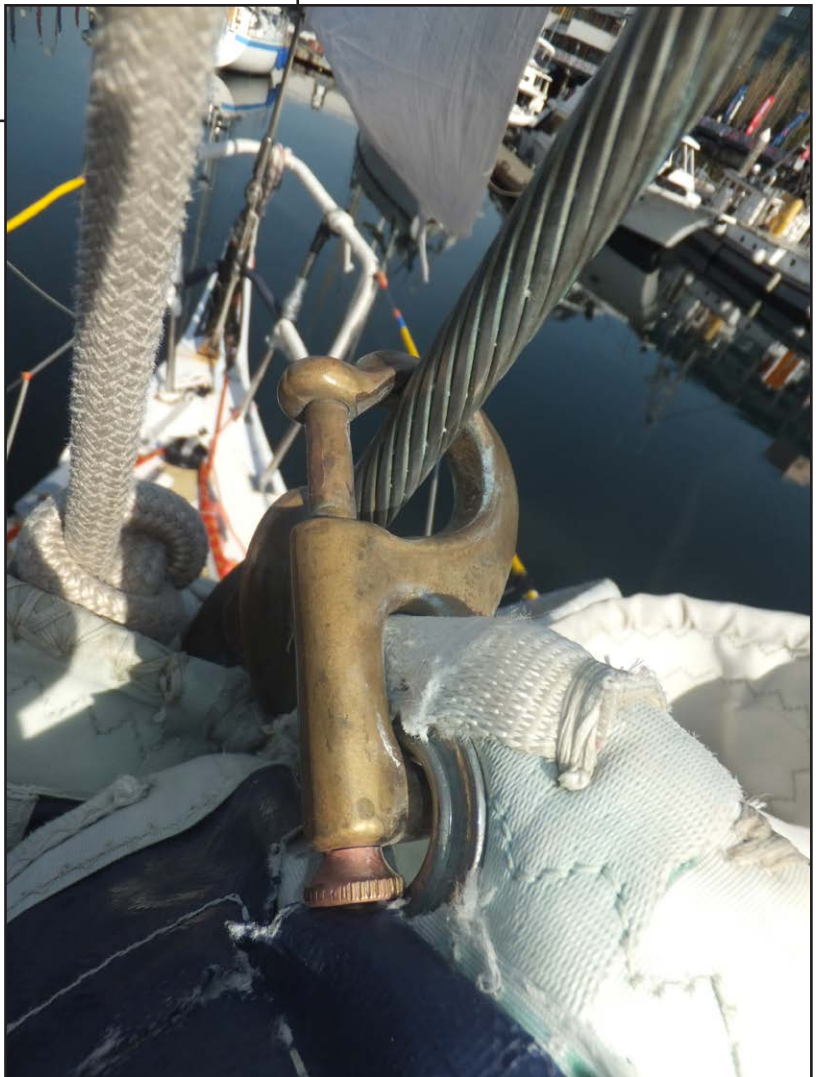
Figure 3: Piston hank used to attach headsail luff to forestay
